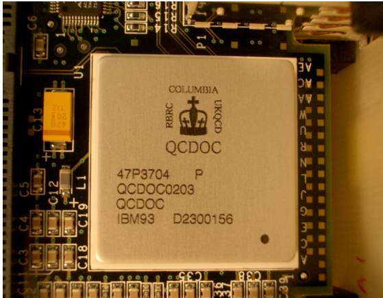
An ASIC (node). ~5 Watt at 400MHz
