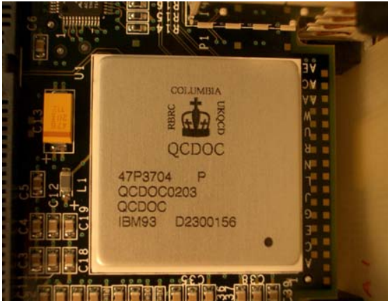
An ASIC (node). ~5 Watt at 400MHz
