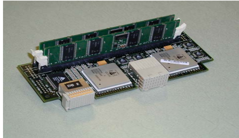
A daughterboard with two nodes and the vertically mounted DDR SDRAMs (128MB at BNL)
