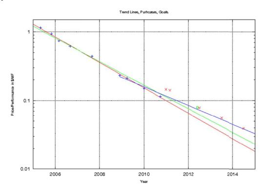
Here, the red line is the least-squares fit to the clusters purchased between 2005 and 2011, shown as blue "+" symbols. The red "X" symbols are goals used in the project plan. The green "o" is the JLab 12s cluster. The green line is the fit to the points from 2005 through 12s. The blue line is the fit to the points from late 2008 through 12s.
