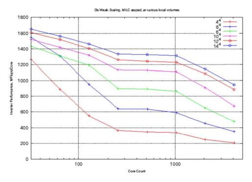
The USQCD cluster ratings use job sizes of 128. For local volumes of 14<sup>4</sup>, performance per core of the asqtad inverter on jobs from 128 through 4096 cores on Ds is as follows:
