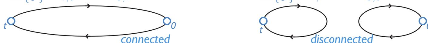
The diagram illustrates the decomposition of the correlator into connected and disconnected parts. On the left, a single loop with vertices labeled  $t$  and  $0$  is shown, labeled "connected". On the right, two separate loops are shown: one with vertices labeled  $t$  and  $t$ , and another with vertices labeled  $0$  and  $0$ , labeled "disconnected".
